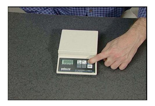
First turn the scale on. The scale must remain on while changing the rate chip to retain the memory.
